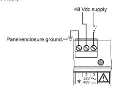
Note: connection to the IQ4E is polarity independent.
