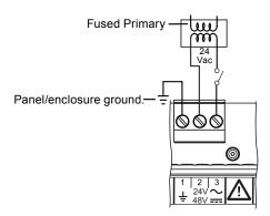
The local earth terminal (1) must be earthed (grounded) at the controller. The 24 V supply must include a suitably rated switch in close proximity and be clearly marked as the disconnecting device for the unit. Do not position the equipment so that the disconnecting device is difficult to operate.
