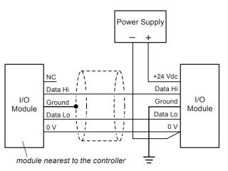
*Important*: The 0 V connection must be made when an external supply is used and the 0 V line must be continuous for the entire length of the I/O bus.
