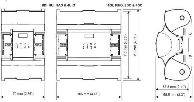
IQ4/IO/.. Modules Data Sheet TA201341 Issue 4, 17-Jun-2016. Applies to I/O Module Fimware v2.20.
