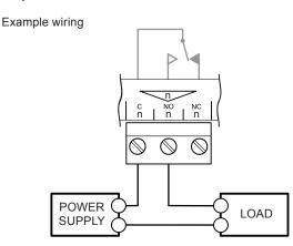
The relay contacts close (i.e. NO makes with C) when the output channel is ON.
