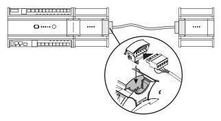
Note: The IQ4/IC/ADPT cable adapter includes non-replaceable fuses and Transient Voltage Suppression diodes that protect the I/O bus from over-current and over-voltage conditions caused by electrical transients or incorrect wiring.
