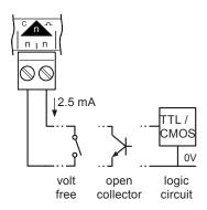
The volt free contact has a nominal wetting current of 2.5 mA. The input is ON when the contact is closed.
