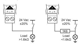
In the above example the input will be ON when the load is powered. If the load impedance is less than 1.6 k $\Omega$  (e.g. a filament lamp or relay coil) then a 1.6 k $\Omega$  resistor must be fitted in series with the input.
