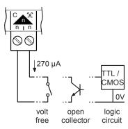
The volt free contact has a nominal wetting current of 270  $\mu A.$  The input is ON when the contact is closed.
