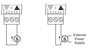
In loop powered mode the output terminal  $rac{1}{2}$  can source up to a maximum of 20 Vdc to power the sensor.
