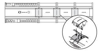
Note: Rigid interconnectors cannot be used between IQ4/IO modules and XCITE/IO modules or an IQ3/XCITE controller. In such cases a cabled interconnection must be used (see below).
